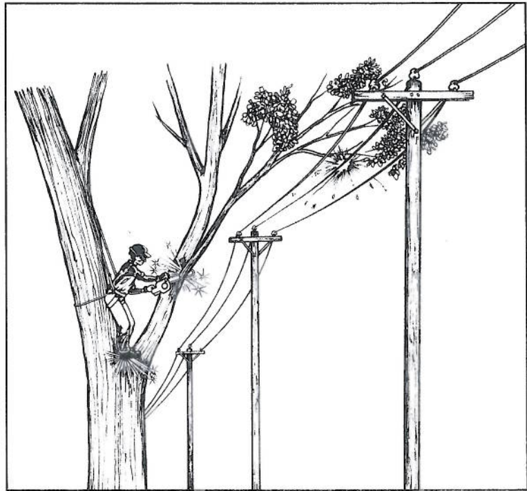
Figure 2. Indirect contact with energized conductors can be as deadly as direct contact.
