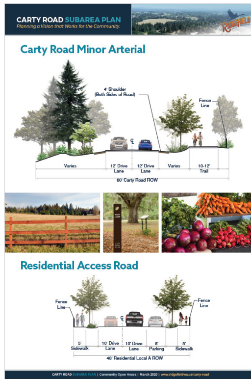
Figure 6. Proposed Street/Road Cross Sections
