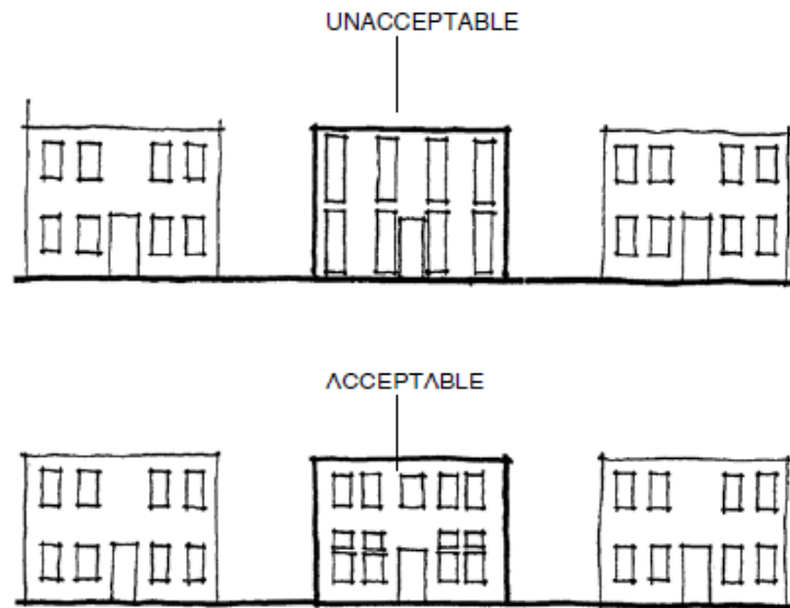
Referring to the pattern and organization of windows on existing structures can achieve a higher level of compatibility.
