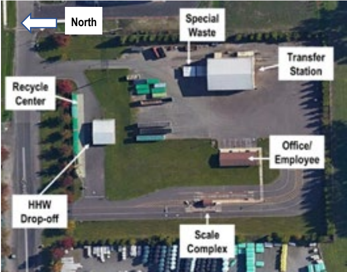
Figure 20: Current Washougal Site Plan
