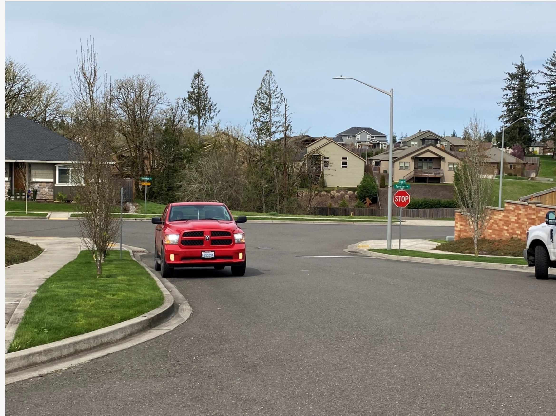
Parked vehicle on south side (no parking now, would be allowed with “flip” of parking zones). Partial sight distance obstruction turning from Meadowlark Loop.
