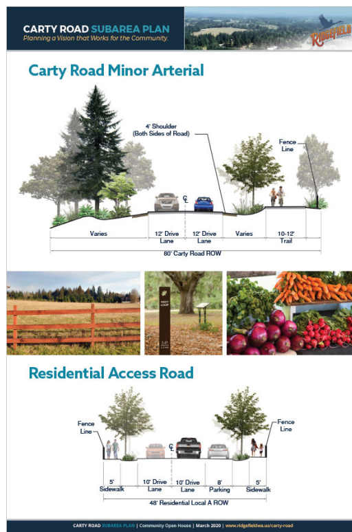
Figure 6. Proposed Street/Road Cross Sections
